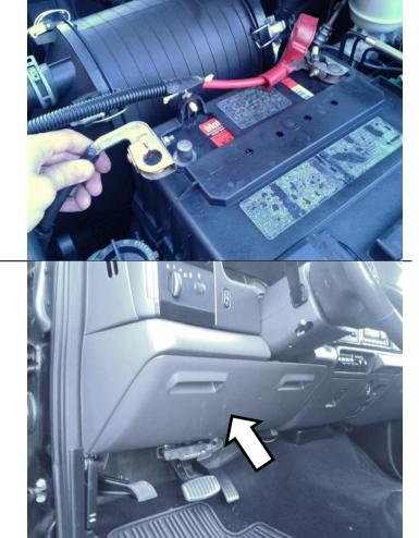
Remove the knee bolster below the steering column.
