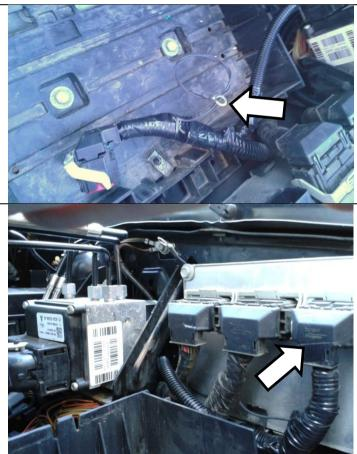
Reinstall the connector into the PCM.
